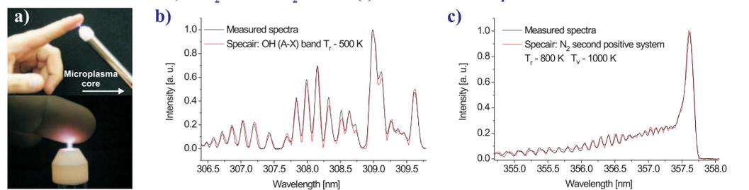
Photos of Ar microplasma (a), comparison of the measured and simulated in Specair program emission spectra of OH (A-X) band (b) and N<sub>2</sub> second positive system (c). 3600 g/mm grating,  $P_{abs} = 10$  W, Ar flow rate - 10 l/min. The observation area within Ar microplasma: core of the visible part of column. MmPS with the MACOR ceramic tip.
