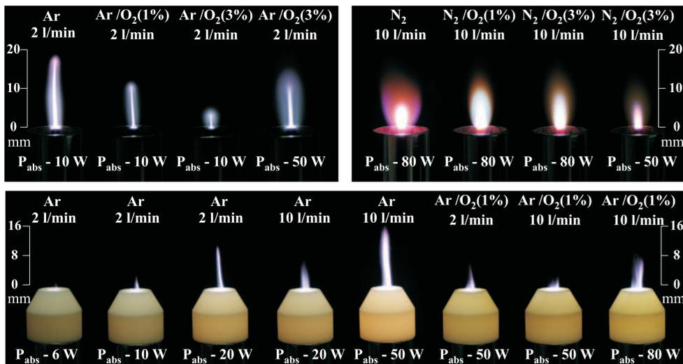
The photos of the microwave microplasma for various operating gases. MmPS without a tip and with the MACOR ceramic tip.
