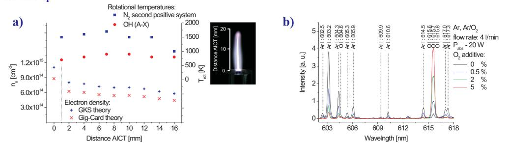
Electron number density  $n_e$  and rotational temperatures of OH and N<sub>2</sub> as a function of distance above the inner conductor top (AICT) in Ar microplasma column.  $P_{abs} = 10$  W, Ar flow rate - 2 l/min (a). Influence of O<sub>2</sub> additive on emission spectra at 602-618 nm (4 mm above inner conductor top).  $P_{abs} = 20$  W, Ar, Ar/O<sub>2</sub> flow rate 4 l/min (b). MmPS without a tip.
