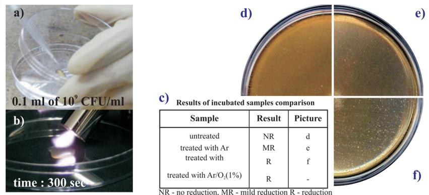
Preliminary test with *Escherichia coli* K-25 bacteria. Placing of 0.1 ml dilution (10<sup>9</sup> CFU/ml) on sterile Petri dish (a). Sample treated with microplasma at microwave absorbed power of 10 W and flow rate of 4 l/min (b). Results confirmed bacteria reduction in treated samples (c): uniform bacteria colony distribution (d) in the untreated sample and spotted bacteria colony distribution in Ar (e) and Ar/O<sub>2</sub> (f) microplasma treated samples.
