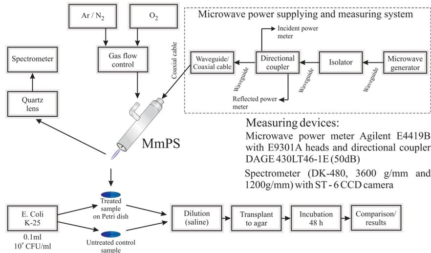
Diagram of the experimental setup for diagnostics of low-temperature microplasma for bio-sterilization.
