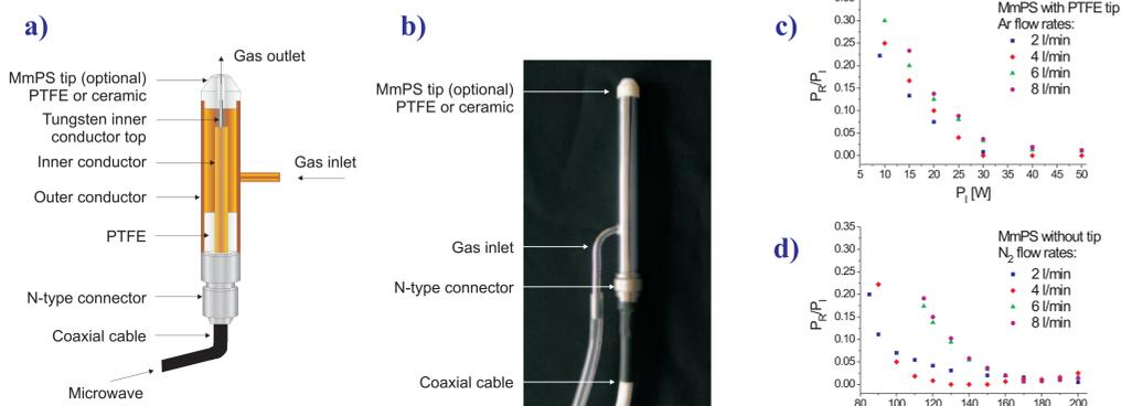
The sketch (a) and the photo (b) of the coaxial-line-based MmPS with tungsten inner conductor top. The reflection coefficient  $P_R/P_I$  ( $P_R$  - reflected microwave power) as a function of the incident microwave power  $P_I$  for the different argon (c) and nitrogen (d) flow rate.
