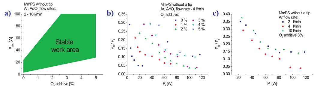
Required absorbed microwave powers for stable microplasma generation for different O<sub>2</sub> additive (a). Ar, Ar/O<sub>2</sub> flow rate from 2 l/min to 10 l/min. The reflection coefficient  $P_R/P_I$  ( $P_R$  - reflected microwave power) as a function of the incident microwave power  $P_I$  for the different O<sub>2</sub> additive at Ar, Ar/O<sub>2</sub> flow rate of 4 l/min (b) and for different flow rates of Ar, Ar/O<sub>2</sub> at 3% of O<sub>2</sub> additive (c). MmPS without a tip.
